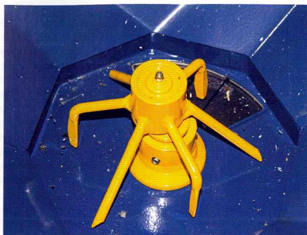
...and double bearing agitators. Latter are better for variable rate spreading.
